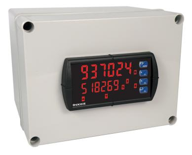
**DESCRIPTION** A low-cost, compact, NEMA 4X enclosure that will house one PRD1000 meter. The cover is held in place with four screws. A ½" conduit hole is provided.
